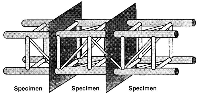
NOTE 1—Each specimen comprises nominally one third of the total surface area of the article. A minimum of five measurements should be made within the volume of each specimen, as widely dispersed within that volume as is practical, so as to represent as much as possible, the general coating thickness within that specimen volume.
